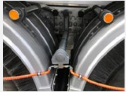
Chassis Pole and Tee Tap
